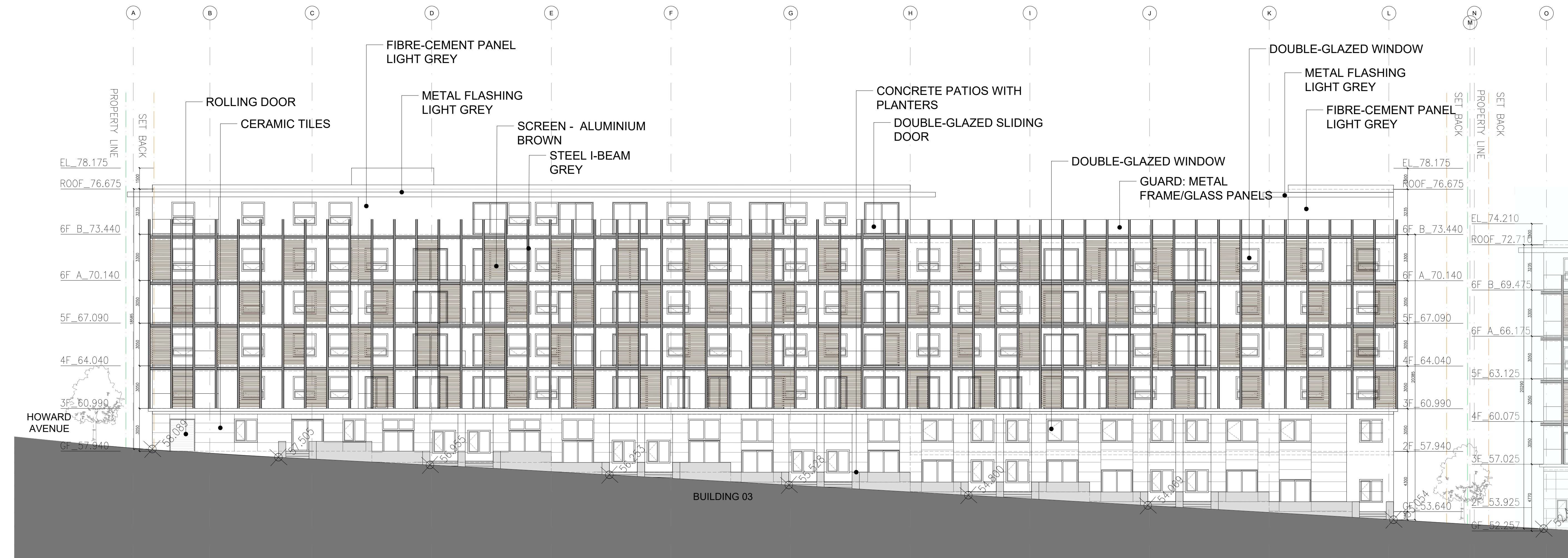
2 SOUTH ELEVATION - BLDG 3 A3.03 1:150
